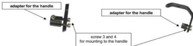
**Step 2:** Remove screw 1 and 2 from adapter, insert the adapter into the battery tube, after that screw in screw 1 and 2 into the holes of the battery tube
