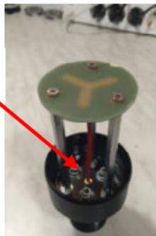
**IMPORTANT !** Make sure, that the battery will not be damaged at the border of battery holder during the mounting and dismounting.
